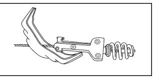
Tilt the tire toward the vehicle. Separate the tire/ wheel retainer (G) from the guide pin. Pull the pin through the center of the wheel. Tilt the retainer down through the center wheel opening.
